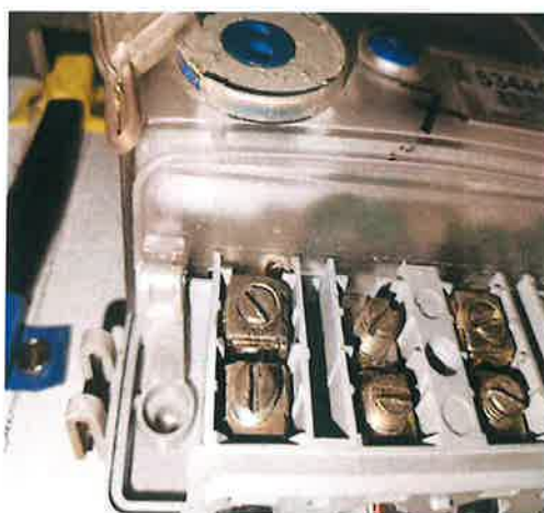
Meter tampered by making hole
